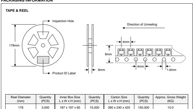
Note: 1. Anti-static plastic reel, white, water clear or blue color. Inspection hole might be varied in different alignment.
