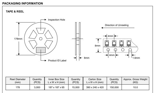
Note: 1. Anti-static plastic reel, white, water clear or blue color. Inspection hole might be varied in different alignment.
