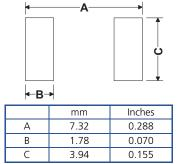
Soldering temperature should be 260°C for a maximum of 10 seconds.
