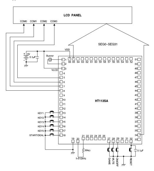
Note: The IC substrate should be connected to VSS in the PCB layout artwork.
