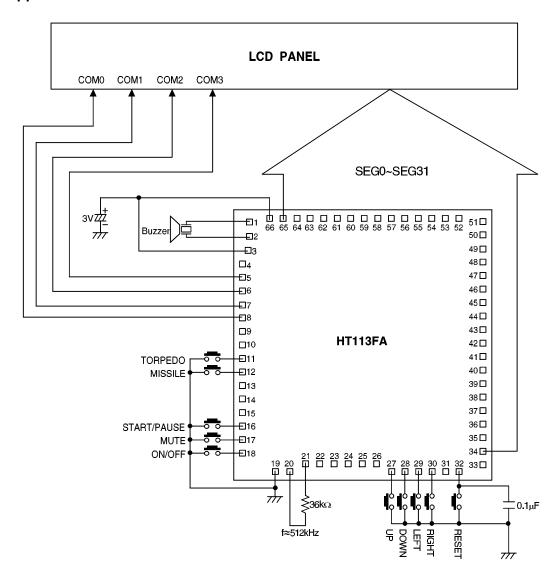
Note: The IC substrate should be connected to VSS in the PCB layout artwork.
