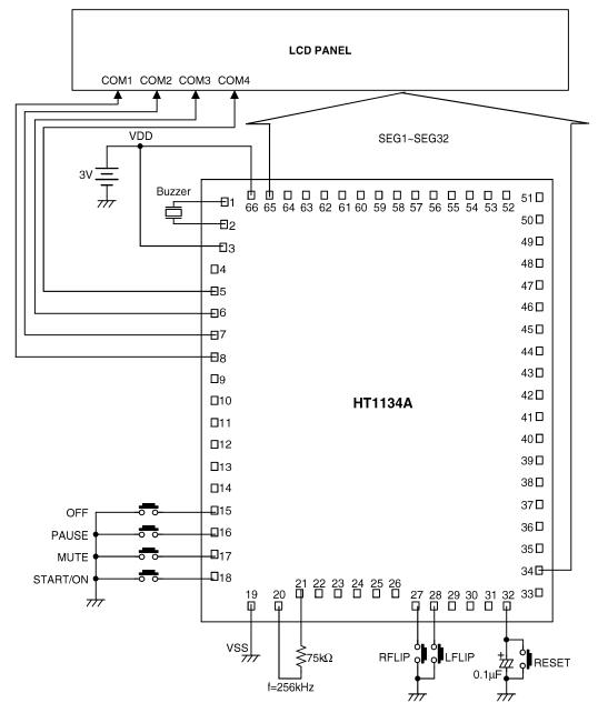
Note: The IC substrate should be connected to VSS in the PCB layout artwork.
