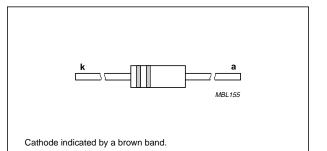
Fig.1 Simplified outline (SOD125A) and symbol.
