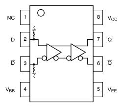
Figure 1. Logic Diagram and Pinout Assignment
