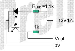
Typical installation: Customer has to select suitable resistors for their chosen supply voltage. Forward voltage of LED is 1.3V and LED current should be 10mA (depending on application liquid). Therefore, for a supply of Vs:
