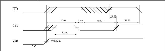
Note : The  $t_{C2HL}$  specifies from CE2 Low to High transition after  $V_{DD}$  reaches specified minimum level.  $\overline{CE1}$  must be brought to High prior to or together with CE2 Low to High transition.
