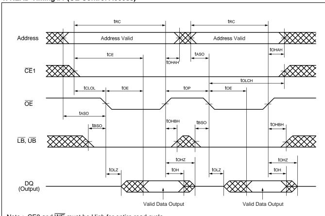
Note : CE2 and  $\overline{\text{WE}}$  must be High for entire read cycle. Either or both  $\overline{\text{LB}}$  and  $\overline{\text{UB}}$  must be Low when both  $\overline{\text{CE}}$ 1 and  $\overline{\text{OE}}$  are Low.
