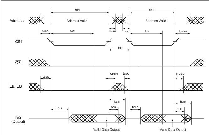
Note : CE2 and  $\overline{\text{WE}}$  must be High for entire read cycle. Either or both  $\overline{\text{LB}}$  and  $\overline{\text{UB}}$  must be Low when both  $\overline{\text{CE}}$ 1 and  $\overline{\text{OE}}$  are Low.
