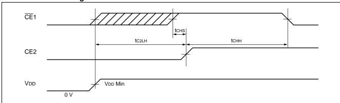
Note : The  $tc_{2LH}$  specifies after  $V_{DD}$  reaches specified minimum level.
