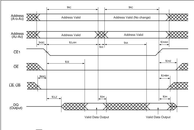
Note : CE2 and  $\overline{\text{WE}}$  must be High for entire read cycle.
