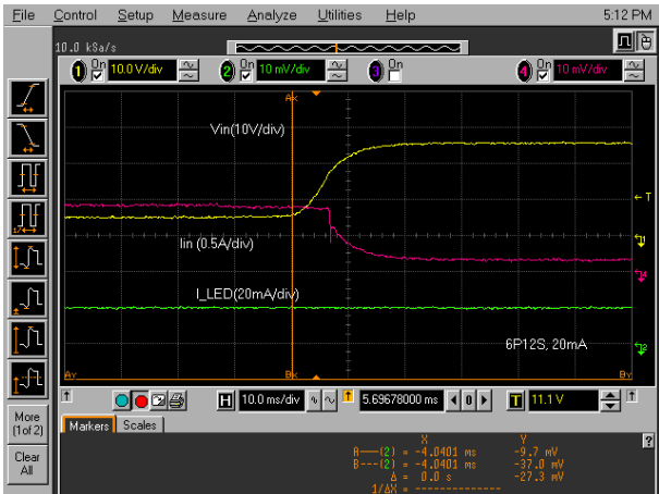
FIGURE 13. LINE REGULATION WITH V_{IN} CHANGE FROM 6V TO 26V, V_{IN} = 12V , 4P12S AT 20mA/CHANNEL
