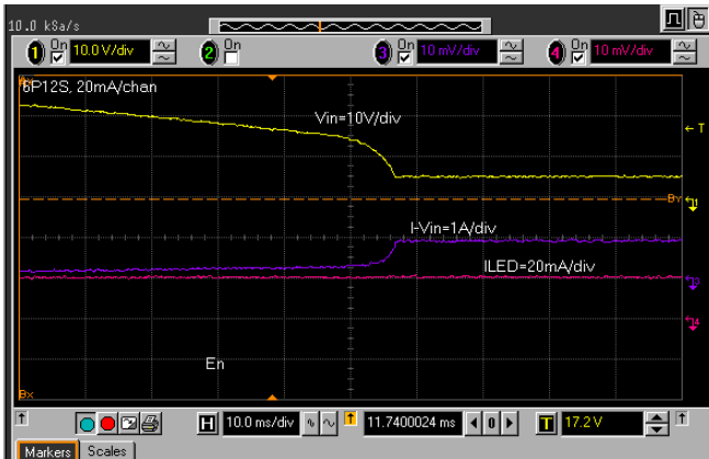
FIGURE 16. LINE REGULATION WITH V_{IN} CHANGE FROM 26V TO 6V FOR 6P12S AT 20mA/CHANNEL
