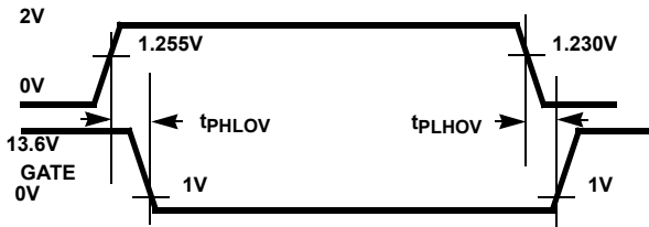
FIGURE 3A. OV TO GATE TIMING
