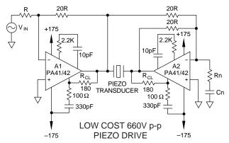
Two PA41/42 amplifiers operated as a bridge driver for a piezo transducer provides a low cost 660 volt total drive capability. The  $R_N C_N$  network serves to raise the apparent gain of A2 at high frequencies. If  $R_N$  is set equal to R the amplifiers can be compensated identically and will have matching bandwidths.
