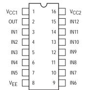
Pin assignment is for Dual–in–Line Package. For PLCC pin assignment, see the Pin Conversion Tables on page 18 of the ON Semiconductor MECL Data Book (DL122/D).
