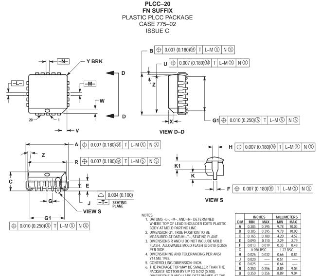
6. THE PACKAGE TOP MAY BE SMALLER THAN THE PACKAGE BOTTOM BY UP TO 0.012 (0.300). DIMENSIONS R AND U ARE DETERMINED AT THE OUTERMOST EXTREMES OF THE PLASTIC BODY EXCLUSIVE OF MOLD FLASH, TIE BAR BURRS, GATE BURRS AND INTERLEAD FLASH, BUT INCLUDING ANY MISMATCH BETWEEN THE TOP AND BOTTOM OF THE PLASTIC BODY.
