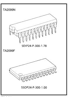
Weight: SDIP24-P-300-1.78: 1.2 g (typ.) SSOP24-P-300-1.00: 0.31 g (typ.)
