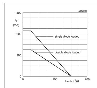
Device mounted on an FR4 printed-circuit board.
