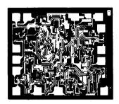
Type ULN-3809A exhibits 35 dB suppression of the 19-kHz pilot and 45 dB rejection of the regenerated 38-kHz subcarrier at demodulator output terminals. Stereo channel separation is typically 47 dB. With a composite input signal of 850 mV, total harmonic distortion for the unit is typically 0.06%.
