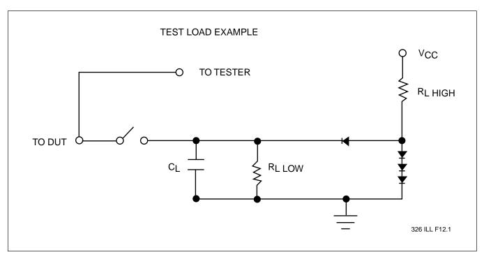
FIGURE 13: A TEST LOAD EXAMPLE
