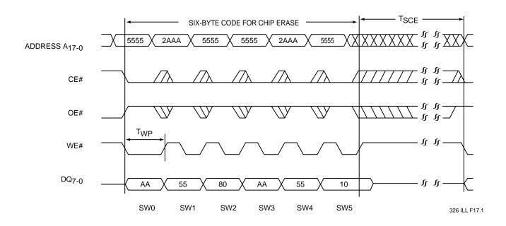
Note: The device also supports CE# controlled chip erase operation. The WE# and CE# signals are interchangeable as long as minimum timings are met. (See Table 10)
