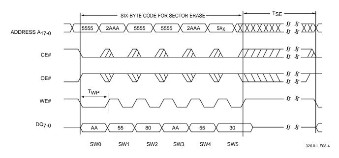
Note: The device also supports CE# controlled sector erase operation. The WE# and CE# signals are interchangeable as long as minimum timings are met. (See Table 10) SA<sub>X</sub> = Sector Address
