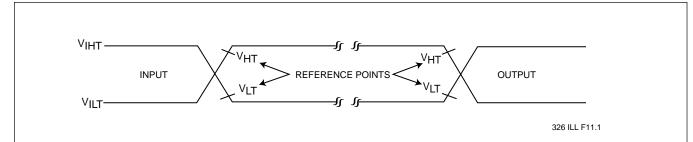
AC test inputs are driven at  $V_{IHT}$  (2.4 V) for a logic "1" and  $V_{ILT}$  (0.4 V) for a logic "0". Measurement reference points for inputs and outputs are  $V_{HT}$  (2.0 V) and  $V_{LT}$  (0.8 V). Inputs rise and fall times (10%  $\leftrightarrow$  90%) are <10 ns.
