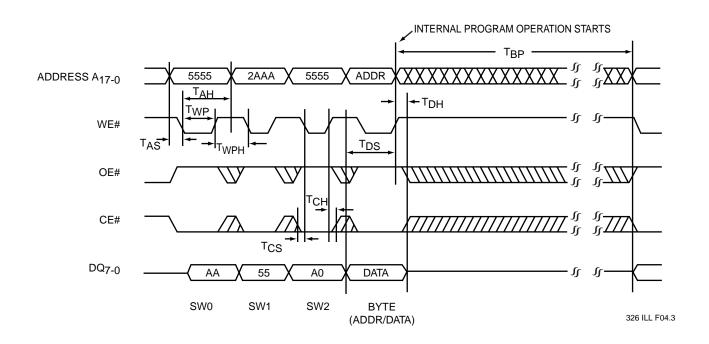
FIGURE 4: WE# CONTROLLED PROGRAM CYCLE TIMING DIAGRAM
