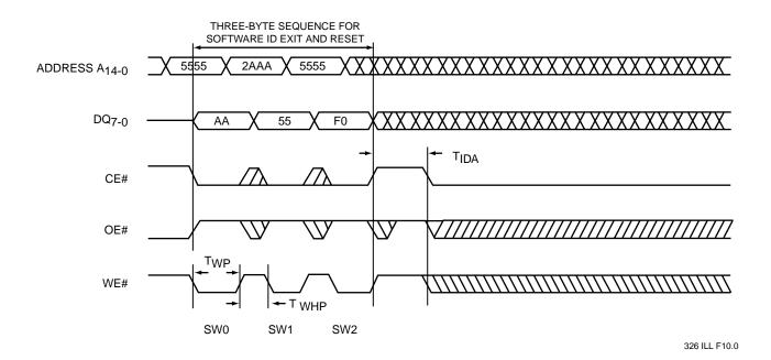
FIGURE 11: SOFTWARE ID EXIT AND RESET
