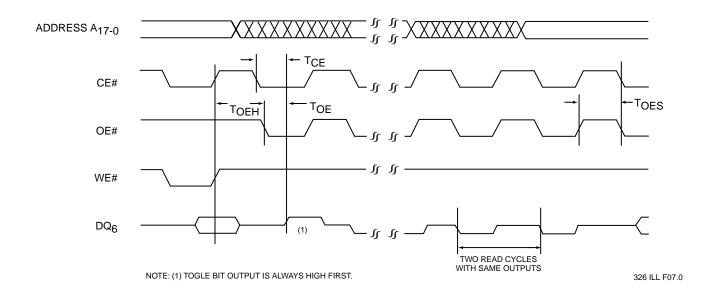
FIGURE 7: TOGGLE BIT TIMING DIAGRAM
