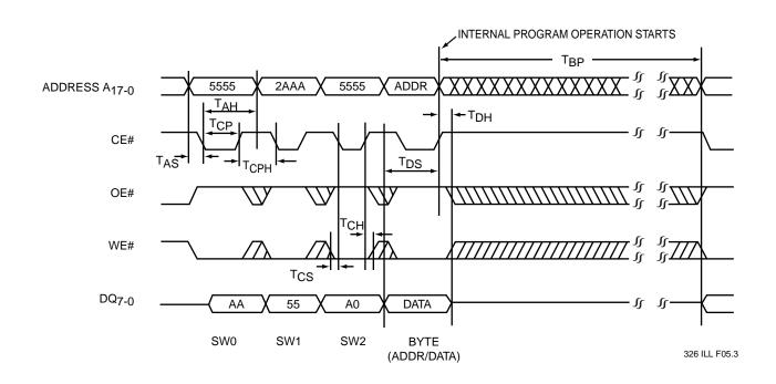
FIGURE 5: CE# CONTROLLED PROGRAM CYCLE TIMING DIAGRAM
