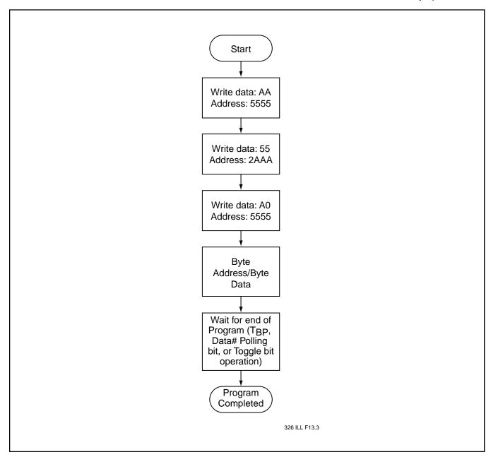
FIGURE 14: BYTE PROGRAM ALGORITHM
