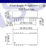
RECOMMENDED FOOTPRINT Top view, grid:2.54mm (0.1 inch) diameter:1.00mm (0.039 inch)
