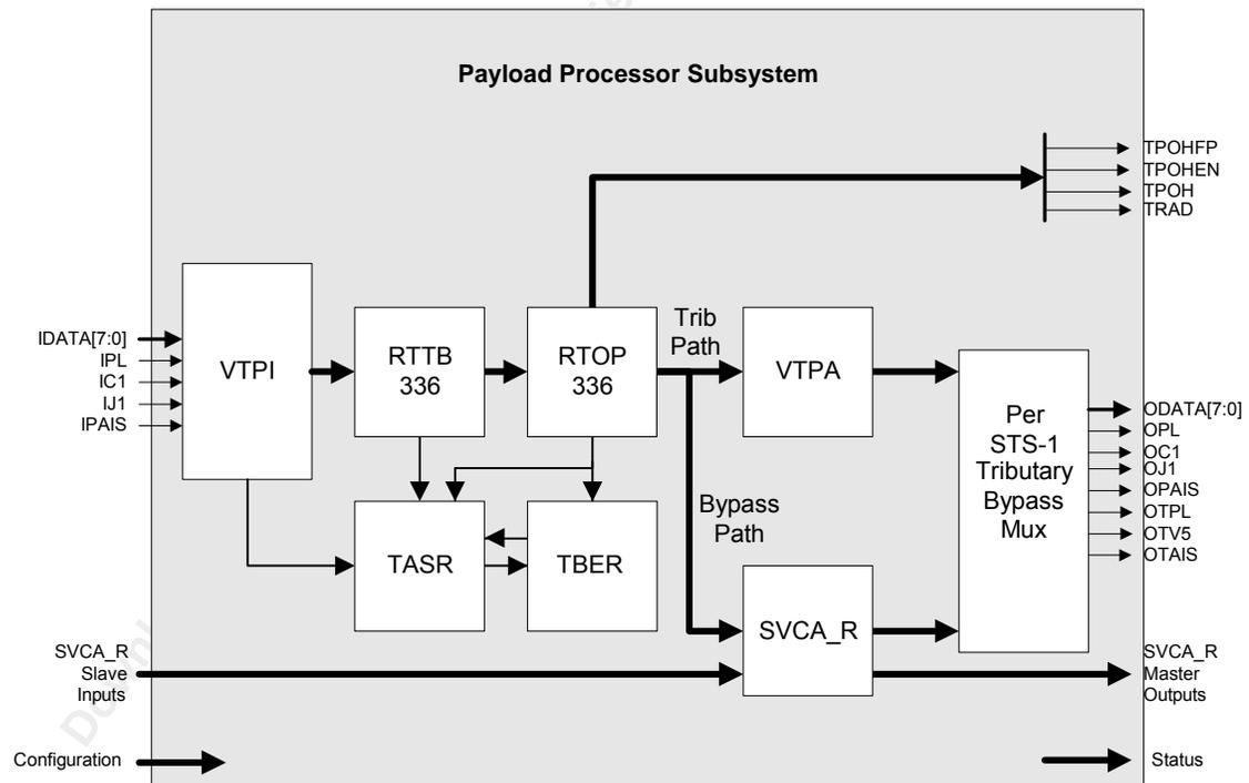
Both paths receive all types of traffic. However, only the bypass path will output valid bypass traffic and only the tributary path will output valid tributary data.
