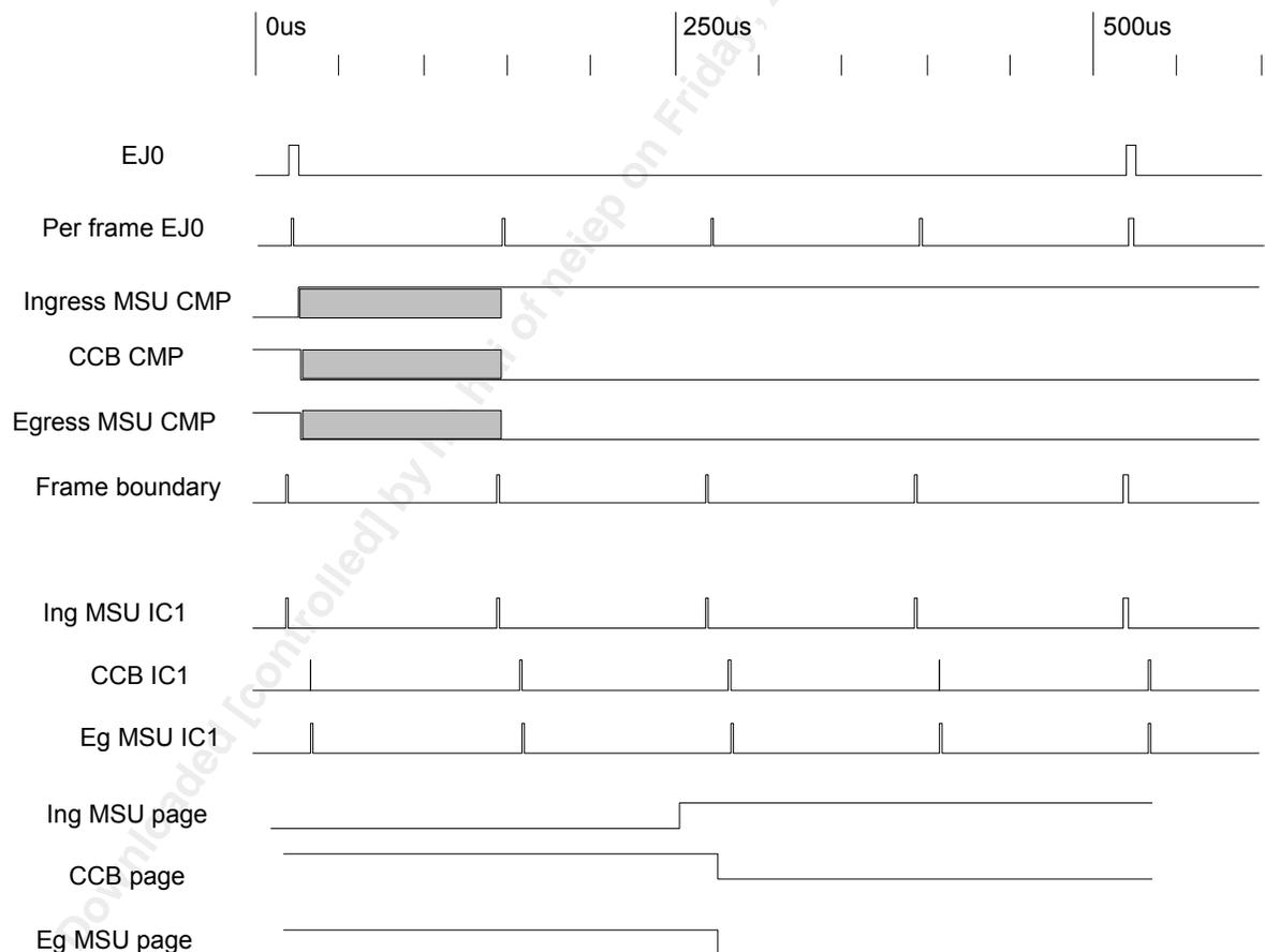
In the figure shown, an internal flywheeled, per frame EJO is shown. Note that CMP should not change for any switch during the per frame EJO pulse, as this is where CMP is sampled for all switches. The IC1(J0) at the input to each switch is shown, along with the location where each switches actual internal CMP changes.
