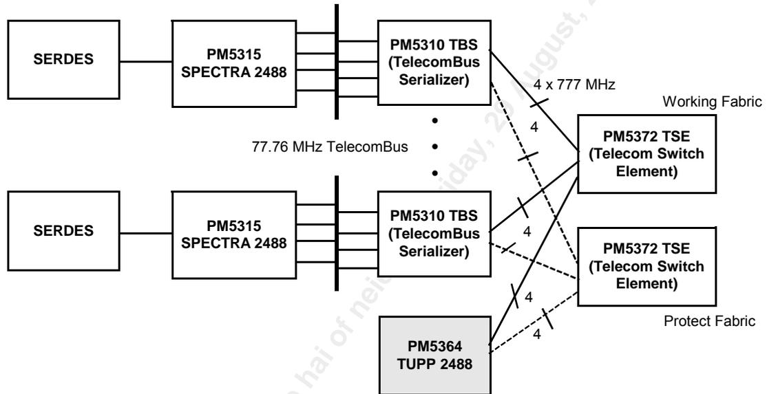
Figure 2 shows how the TUPP 2488 can be used in an OC-48 Add-Drop Multiplexer application.
