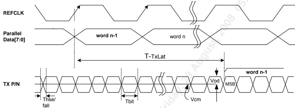
After CML Subsystem processing eight 77.76 MByte/s STS12 channel byte streams are transmitted on the parallel data bus synchronous to REFCLK on the line side (or 16 on the system side)
