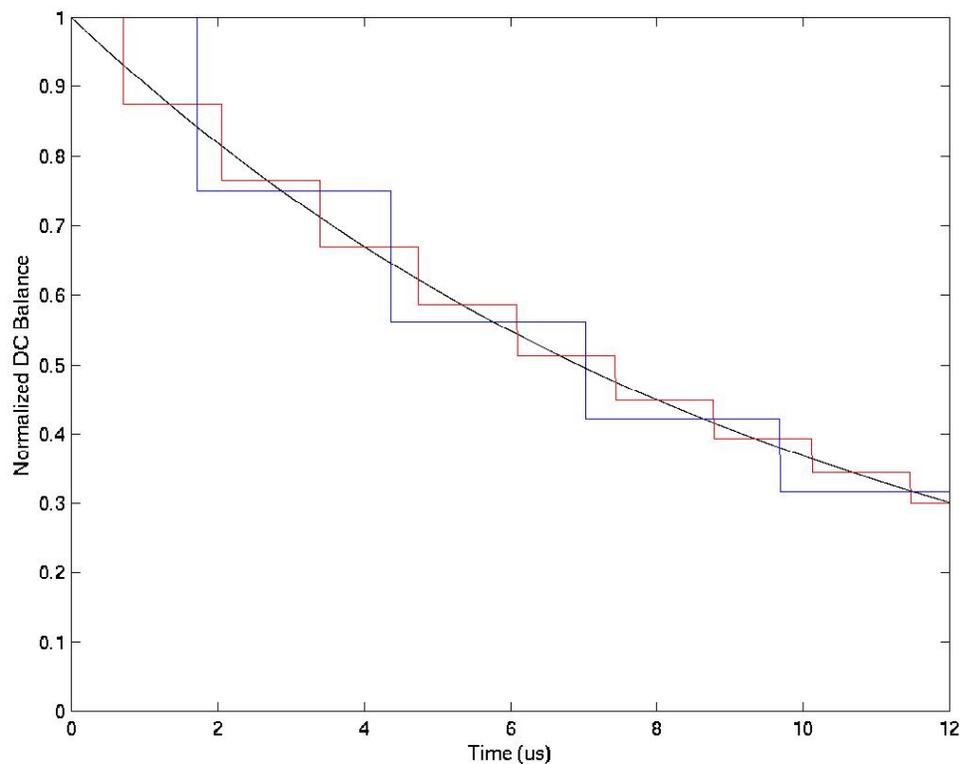
Figure 61 shows the DC balance count over a few frames times with scrambled random data. The decay period is set to 430 and the decay factor is 1/8. Simulations have shown that random data with no bias has maximum DC balance counts of approximately +/-350. With 51% ones and 49% zeros the maximum DC balance counts are around +/-900. Normal SONET data will have a ones density between 49.5% and 50.5% a threshold of 1000 is recommended.
