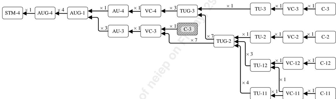
**Figure 22 Supported SONET Frame Structures in Tributary Path**
