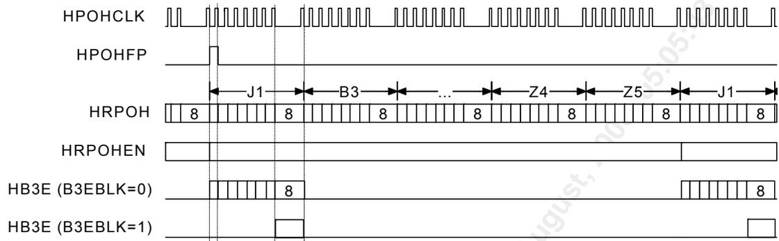
All signals on the HRPOH port are reference to a nominal 20.736 MHz 33% high duty cycle clock (HPOHCLK). HPOHCLK is generated by gapping an internal 25.92 MHz clock. This means that every 2 out of 10 clock edges are skipped to trigger exactly 2,592 clock pulses between each 125  $\mu$ s interval. Note that all signals on the HRPOH port are updated on the falling edges of HPOHCLK.
