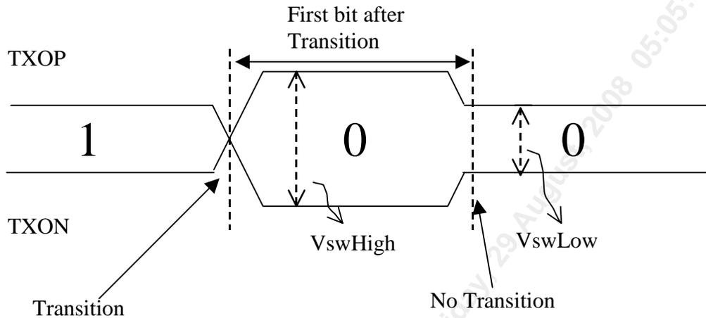
This increased amplitude of bits following transitions helps to counteract frequency dependent attenuation incurred with transmission over PCB traces and cables. The high speed RASIO CML transmitter provides programmable ratios of  $V_{swHigh}$  to  $V_{swLow}$  to provide optimal performance over a wide range of trace lengths.
