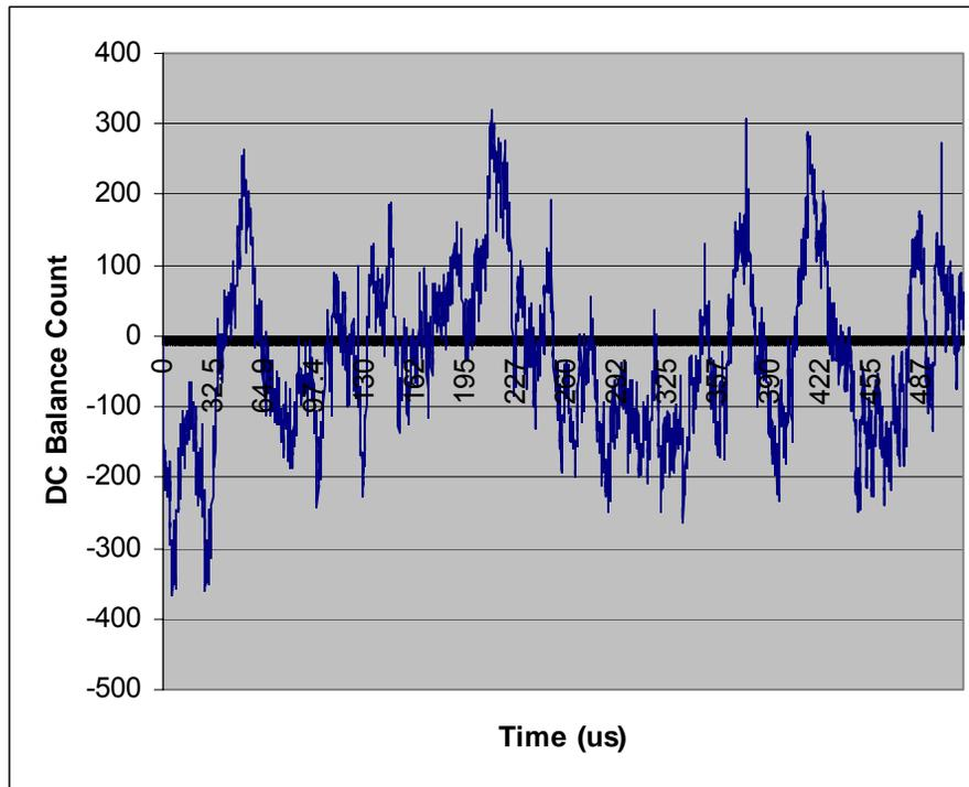
Suggested settings for DECAY\_PER, DECAY\_FAC and DC\_BAL\_THRESH are 108, 1/8, and 500 for 622 Mbit/s links and 430, 1/8, and 1000 for 2.488 Gbit/s links, respectively. The numbers given are to be used guidelines. It is recommended that simulations be run to derive parameters for specific applications.
