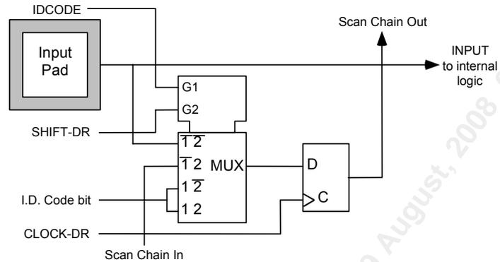
Figure 28 Output Cell (OUT\_CELL)
