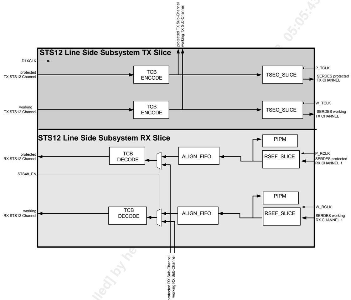
Figure 14 STS-48 CML Line Side Subsystem RX and TX Slices Block Diagram
