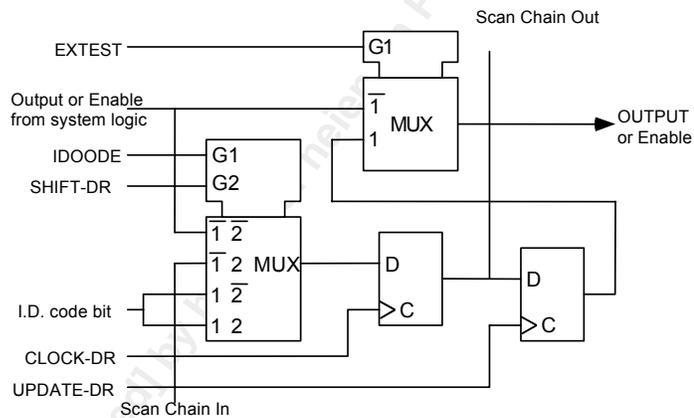
**Figure 29 Bidirectional Cell (IO\_CELL)**
