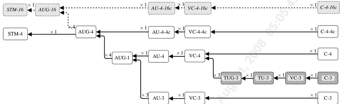
**Figure 24 Supported SONET Frame Structures in Bypass Path**
