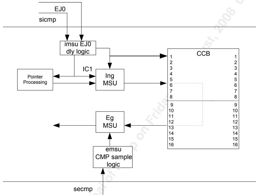
In the above case, the Ingress MSU EJO delay value is 0 clocks. CCB internal CMP sampling delay is delay through Ingress MSU.
