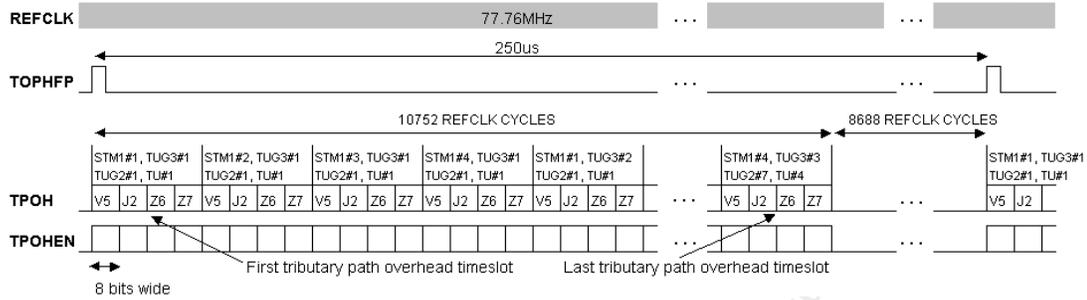
In the event where the STS-12/STM-4 frame contains TU3 tributaries, the TPOH pin will output the 9 path overhead bytes (J1, B3, C2, G1, F2, H4, Z3, Z4, and Z5) on its dedicated timeslots. A summary of the mapping of TU3 overhead byte timeslots to lower order overhead byte timeslots is shown in Table 48. A complete enumeration of the ordering of path overhead bytes presented on the TPOH pin is shown in Table 49.
