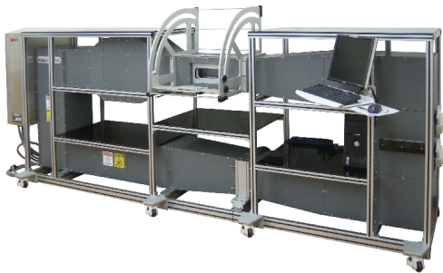
Fig. F: FDK Original Wind Tunnel
