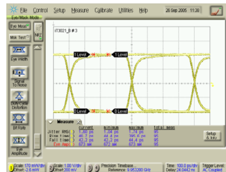
Bit rate: 2.5 Gb/s Vin = +/-100 mVpp, Vout = +/-672 mVpp
