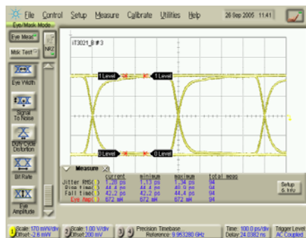
Bit rate: 2.5 Gb/s Vin = +/-200 mVpp, Vout = +/-672 mVpp
