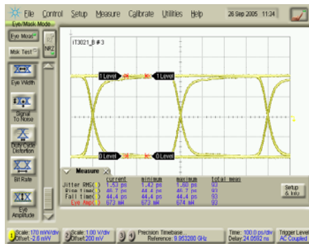
Bit rate: 2.5 Gb/s Vin = +/-50 mVpp, Vout = +/-672 mVpp
