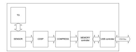
The TG block receives timing signals from the CMOS sensor and generates all the synchronization signals needed inside the SPCA561A, while the CDSP block receives and processes image data from the sensor. The image data is then further compressed by the Compression block and directly transmitted to the USB bus via the USB controller. The detailed function of each block is described in the following subsections.
