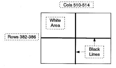
TEST PATTERN FOR IMAGE STICKING TEST
