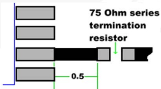
Figure 19. Distance from Device Pin to Series Termination Resistor
