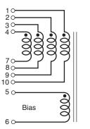
Primary windings to be connected in parallel on the PC board
