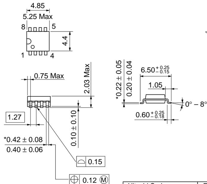
\*Dimension including the plating thickness
