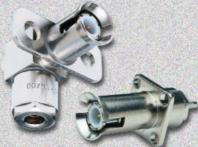
Straight and right angle slide-on panel mounted BNC plugs, clamp and crimp type cable attachment—mate with standard BNC jacks.
