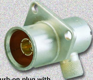
N right angle push-on plug with three-hole flange and crimp cable attachment. Mates with standard type N jack.
