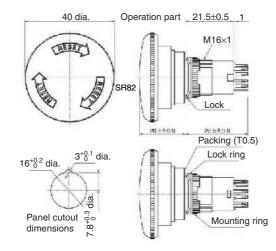
Note: 1. When applying a coating such as paint to the panel, dimensions after the coating must satisfy the specified dimensions.
