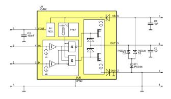
Figure 9: Circuit schematic showing protective devices
