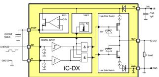
Figure 4: Configuration as High-Side (PNP-Switch)
