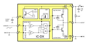
Figure 5: Configuration as Low-Side (NPN-Switch)
