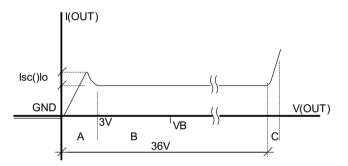
Figure 1: OUT characteristic when Low side active
