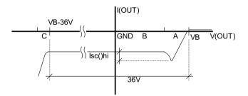
Figure 2: OUT characteristic when high side active
