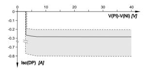
Figure 6: DP short-circuit output current
