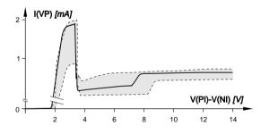
Figure 5: VP supply current, no load
