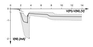
Figure 2: NI input current, I(DP) = -5 mA
