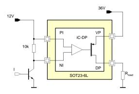
Figure 12: 12 V NPN input control, 36 V output supply
