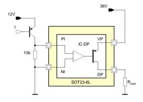
Figure 11: 12 V PNP input control, 36 V output supply
