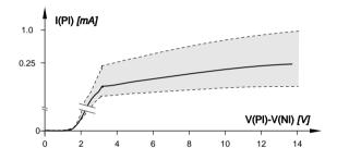
Figure 4: PI input current, load independent
