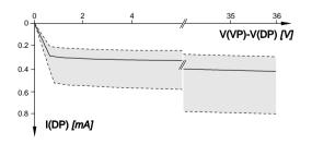
Figure 7: DP output characteristic
