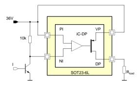
Figure 8: 36 V supply, NPN input control
