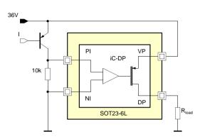
Figure 9: 36 V supply, PNP input control
