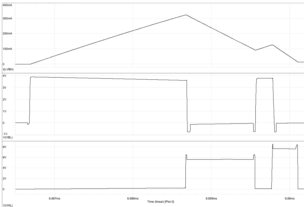
Figure 2: Converter current/voltage characteristics (VB = 4 V)
