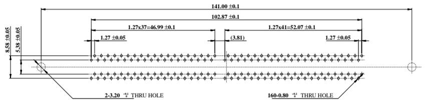
CONTACT & FIXING SCREW HOLE PATTERN
