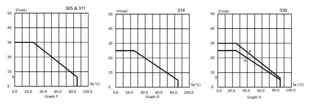
^ = Products must be derated according to the derating information. Each derating graph refers to specific LEDs.
