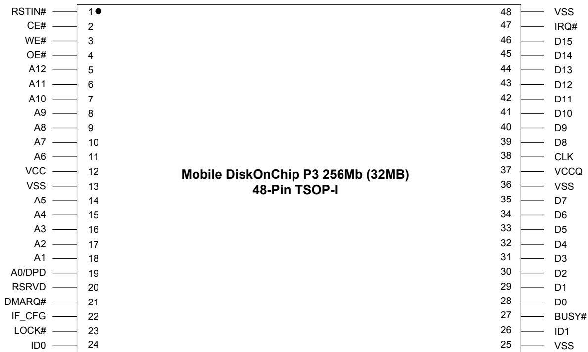
Figure 1: TSOP-I Pinout for Standard Interface (Mobile DiskOnChip P3 256Mb)
