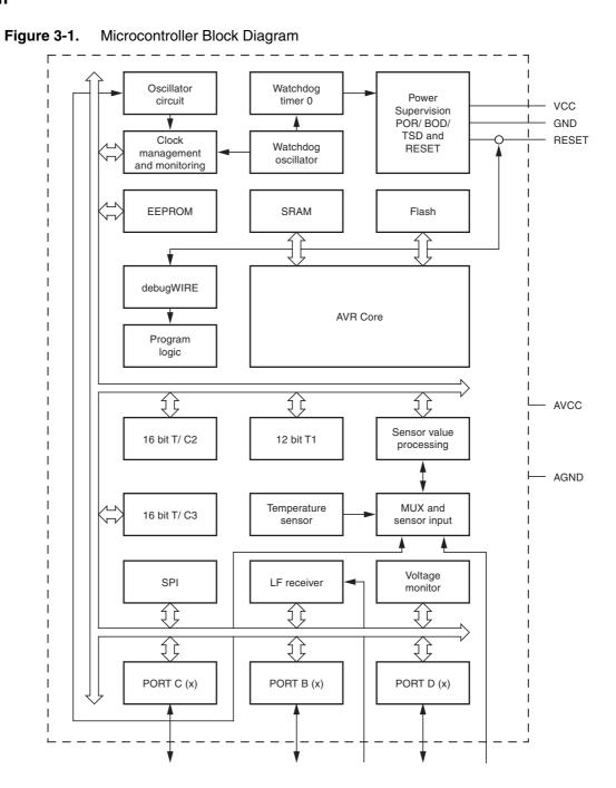
The AVR core combines a rich instruction set with 32 general purpose working registers. All the 32 registers are directly connected to the Arithmetic Logic Unit (ALU), allowing two independent registers to be accessed in one single instruction executed in one clock cycle. The resulting architecture is more code efficient while achieving throughputs up to ten times faster than conventional CISC microcontrollers.
