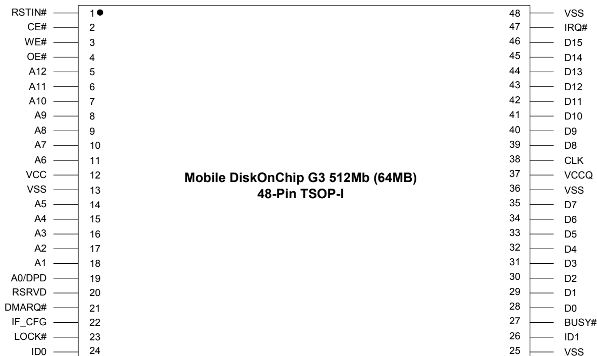
Figure 1: TSOP-I Pinout for Standard Interface (Mobile DiskOnChip G3 512Mb)
