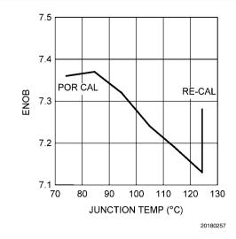
FIGURE 16. ENOB vs. Junction Temperature, 749MHz input
