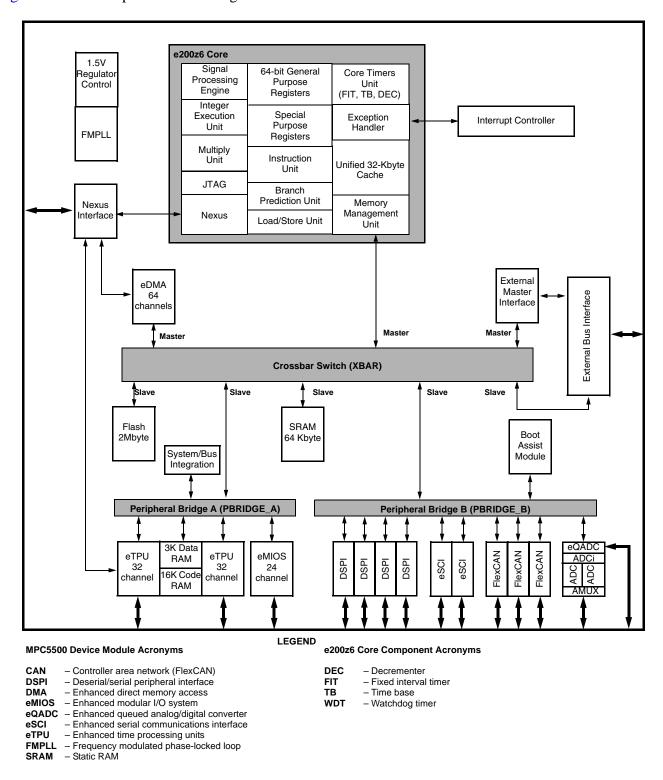
Figure 1. MPC5554 Block Diagram
