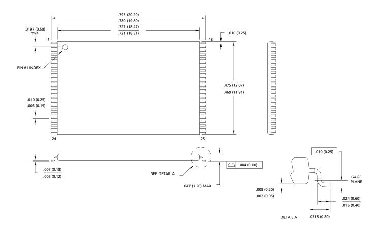
**NOTE:** 1. All dimensions in inches (millimeters)  $\frac{MAX}{MIN}$  or typical where noted.
