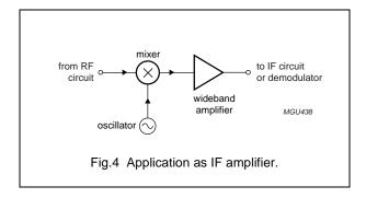
The MMIC is very suitable as IF amplifier in e.g. LNB's. The excellent wideband characteristics make it an ideal building block (figure 4).
