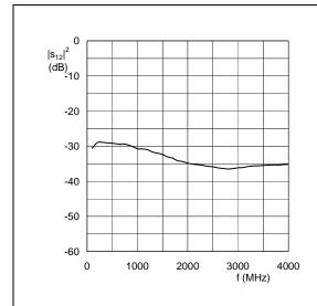
$I_S = 15.9 \text{ mA}$ ;  $V_S = 5.0 \text{ V}$ ;  $P_D = -35 \text{ dBm}$ ;  $Z_O = 50 \Omega$ .
