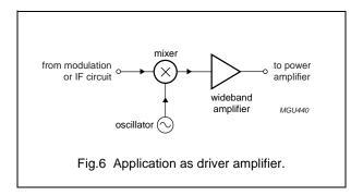
As driver amplifier in the TX path, the good lineair performance and matched in/-output offer quick design (figure 6).
