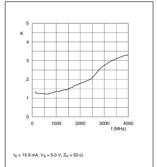
Fig.14 Stability factor as a function of frequency; typical values.
