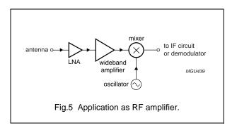
As second amplifier after an LNA, the MMIC offers an easy matching, low noise solution (figure 5).
