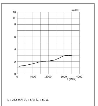
Fig.14 Stability factor as a function of frequency; typical values.
