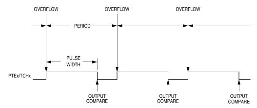
Figure 20-3. PWM Period and Pulse Width
