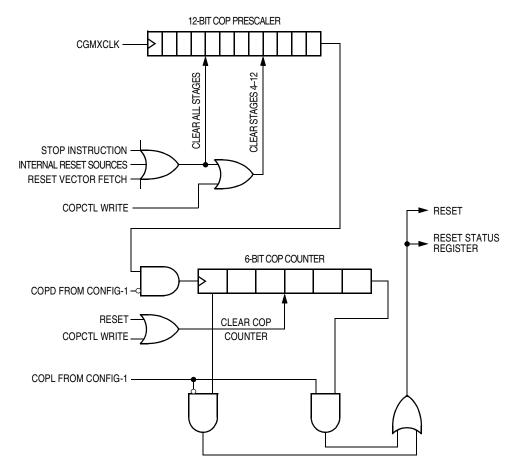
Figure 15-1. COP Block Diagram
