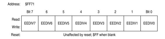
Figure 7-8. EEPROM-2 Divider Non-Volatile Register Low (EE2DIVLNVR)
