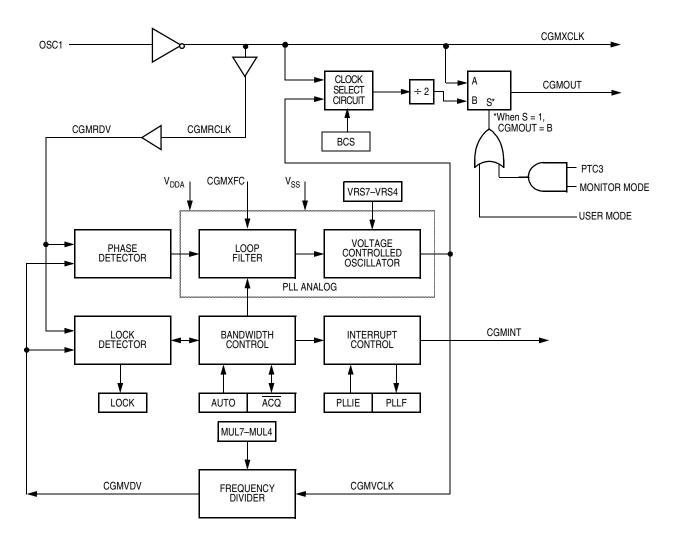
Figure 10-1. CGM Block Diagram
