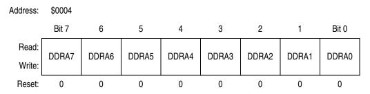
Figure 22-3. Data Direction Register A (DDRA)
