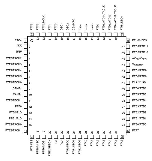
Figure 1-3. MC68HC908AZ60A (64-Pin QFP)
