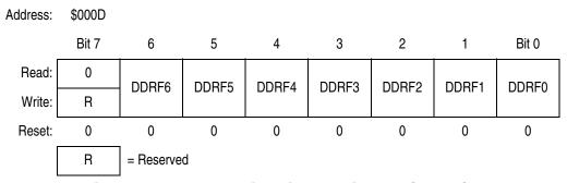
Figure 22-18. Data Direction Register F (DDRF)
