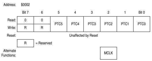
Figure 22-8. Port C Data Register (PTC)
