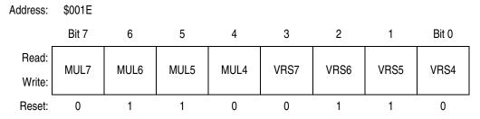
Figure 10-6. PLL Programming Register (PPG)
