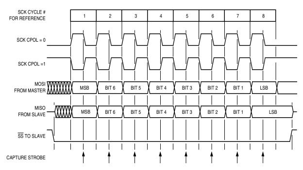
Figure 19-4. Transmission Format (CPHA = 1)
