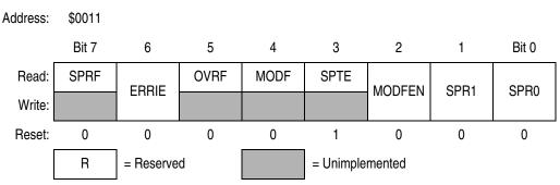
Figure 19-12. SPI Status and Control Register (SPSCR)
