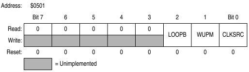
Figure 23-16. Module Control Register (CMCR1)
