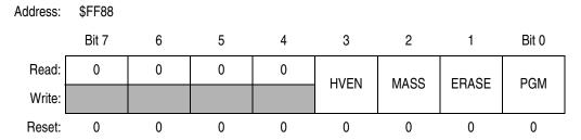
Figure 4-1. FLASH-1 Control Register (FL1CR)
