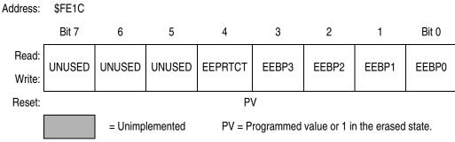
Figure 6-4. EEPROM-1 Nonvolatile Register (EE1NVR)
