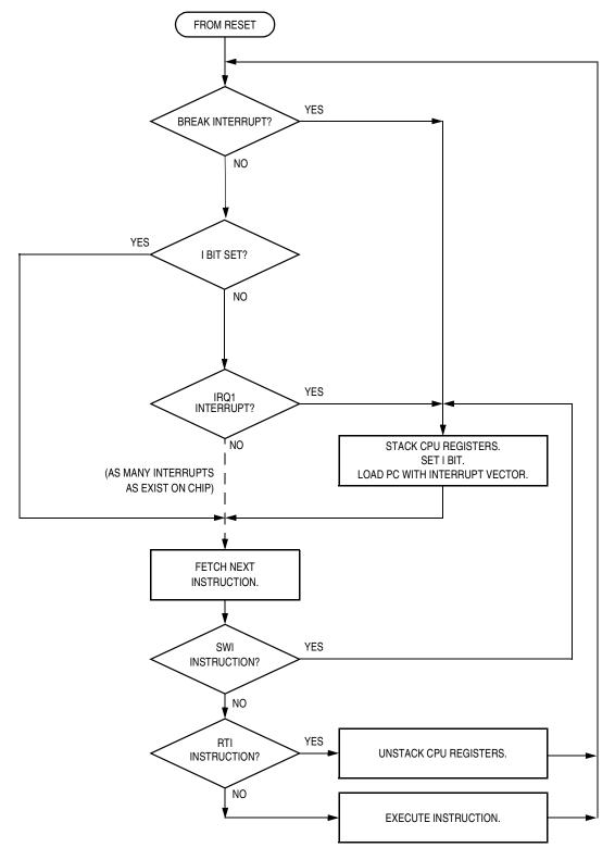
Figure 9-9. Interrupt Processing
