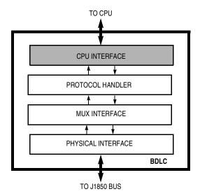
Figure 27-14. BDLC Block Diagram
