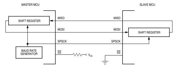
Figure 19-2. Full-Duplex Master-Slave Connections
