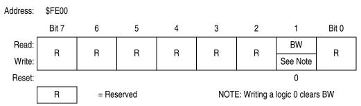
Figure 9-17. SIM Break Status Register (SBSR)
