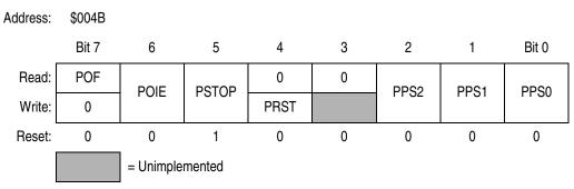
Figure 21-3. PIT Status and Control Register (PSC)
