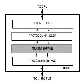
Figure 27-3. BDLC Block Diagram
