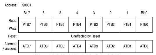
Figure 22-5. Port B Data Register (PTB)
