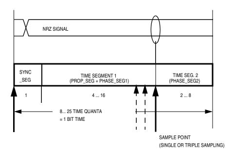
Figure 23-8. Segments within the Bit Time
