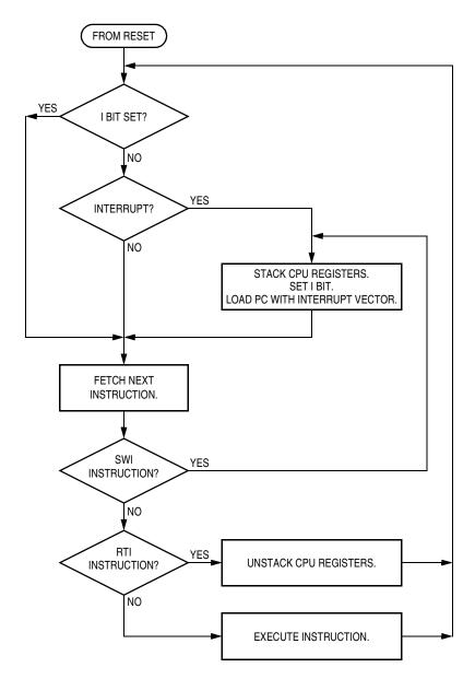
Figure 17-2. IRQ Interrupt Flowchart
