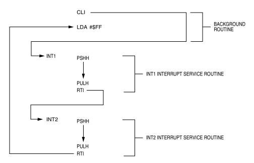
Figure 9-11. Interrupt Recognition Example
