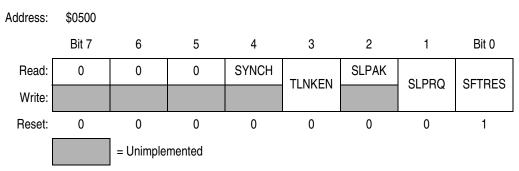
Figure 23-15. Module Control Register 0 (CMCR0)
