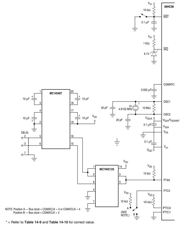
Figure 14-1. Monitor Mode Circuit
