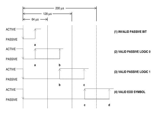
Figure 27-7. J1850 VPW Received Passive Symbol Times
