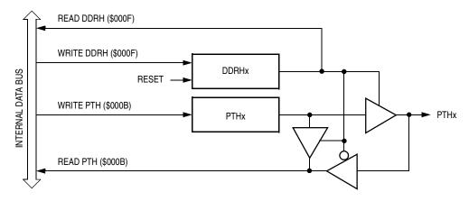
Figure 22-25. Port H I/O Circuit
