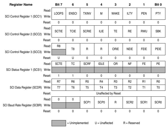
Figure 18-5. SCI Transmitter I/O Register Summary
