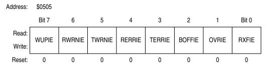
Figure 23-20. Receiver Interrupt Enable Register (CRIER)
