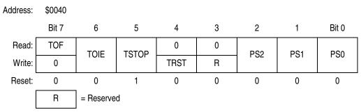
Figure 20-4. TIMB Status and Control Register (TBSC)
