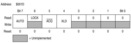
Figure 10-5. PLL Bandwidth Control Register (PBWC)
