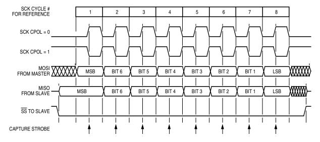
Figure 19-3. Transmission Format (CPHA = 0)
