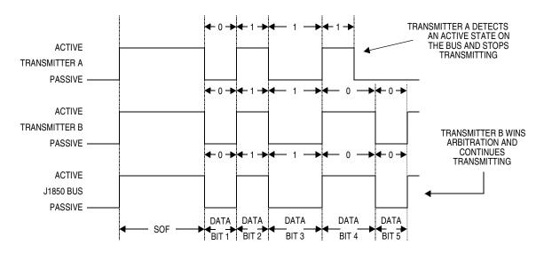
Figure 27-11. J1850 VPW Bitwise Arbitrations
