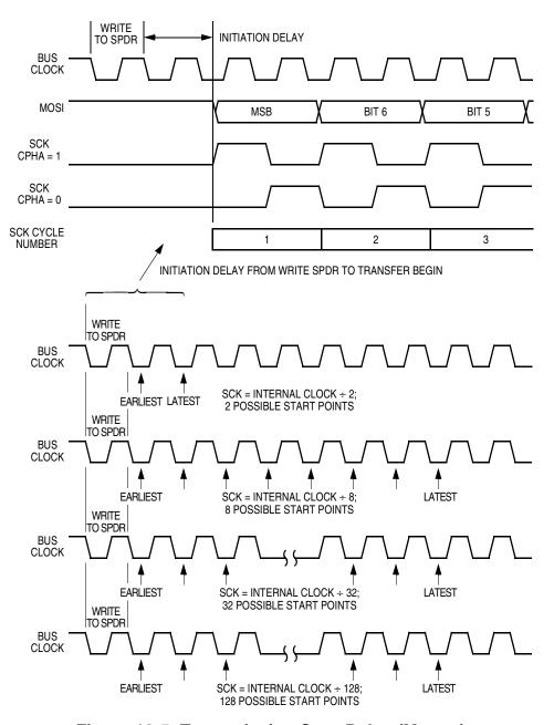
Figure 19-5. Transmission Start Delay (Master)
