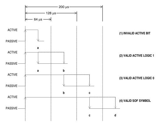
Figure 27-9. J1850 VPW Received Active Symbol Times
