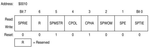
Figure 19-11. SPI Control Register (SPCR)
