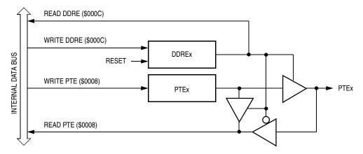
Figure 22-16. Port E I/O Circuit
