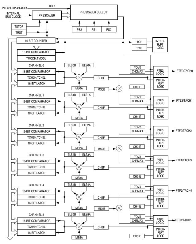
Figure 25-1. TIMA Block Diagram
