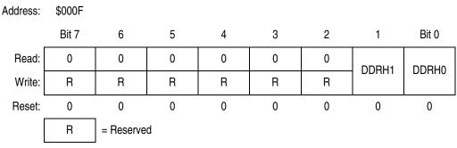
Figure 22-24. Data Direction Register H (DDRH)
