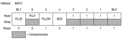
Figure 10-4. PLL Control Register (PCTL)
