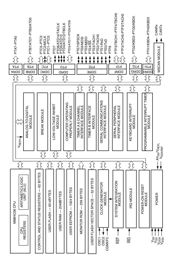
Figure 1-1. MCU Block Diagram for the MC68HC908AZ60A (64-Pin QFP)
