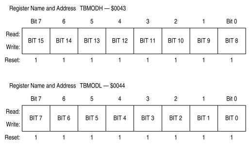
Figure 20-6. TIMB Counter Modulo Registers (TBMODH and TBMODL)
