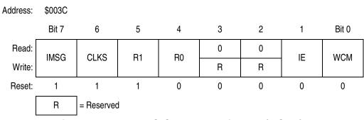
Figure 27-16. BDLC Control Register 1 (BCR1)
