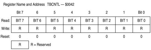
Figure 20-5. TIMB Counter Registers (TBCNTH and TBCNTL)
