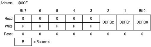
Figure 22-21. Data Direction Register G (DDRG)
