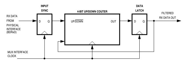
Figure 27-4. BDLC Rx Digital Filter Block Diagram
