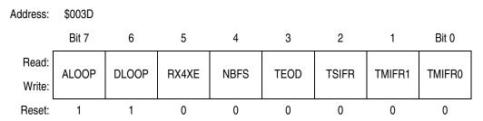
Figure 27-17. BDLC Control Register 2 (BCR2)
