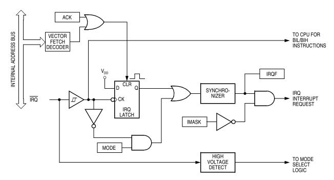
Figure 17-1. IRQ Block Diagram
