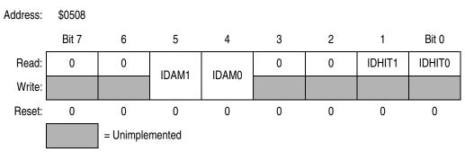
Figure 23-23. Identifier Acceptance Control Register (CIDAC)
