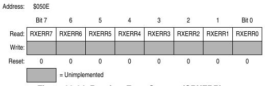
Figure 23-24. Receiver Error Counter (CRXERR)
