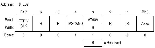
Figure 12-1. Configuration Register (CONFIG-2)
