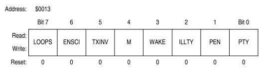
Figure 18-11. SCI Control Register 1 (SCC1)
