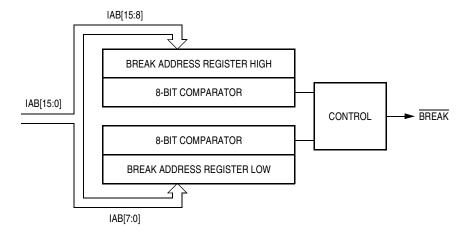
Figure 13-1. Break Module Block Diagram
