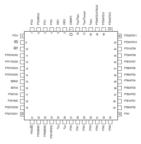
Figure 1-5 shows MC68HC908AS60A 52-pin PLCC pin assignments.
