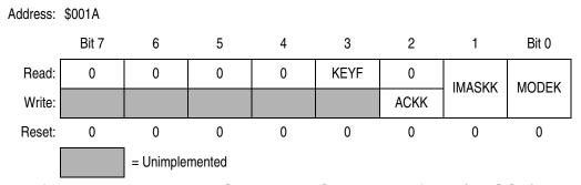
Figure 24-3. Keyboard Status and Control Register (KBSCR)
