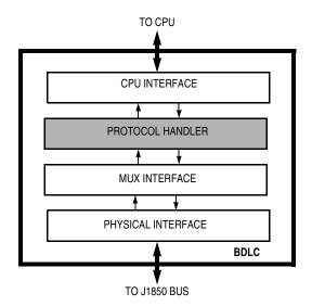
Figure 27-12. BDLC Block Diagram
