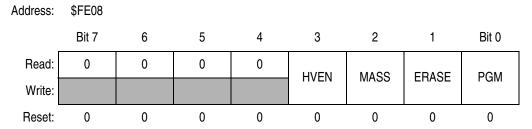
Figure 5-1. FLASH-2 Control Register (FL2CR)
