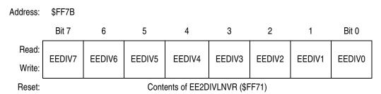
Figure 7-6. EE2DIV Divider Low Register (EE2DIVL)
