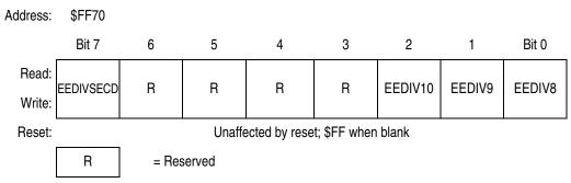
Figure 7-7. EEPROM-2 Divider Non-Volatile Register High (EE2DIVHNVR))
