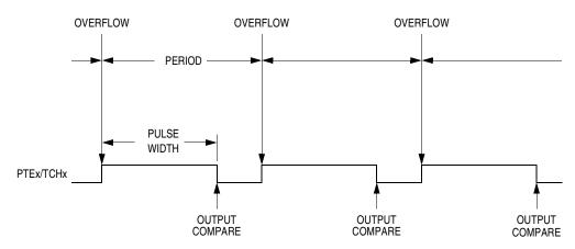
Figure 25-3. PWM Period and Pulse Width
