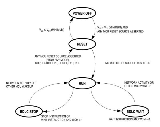
Figure 27-2. BDLC Operating Modes State Diagram
