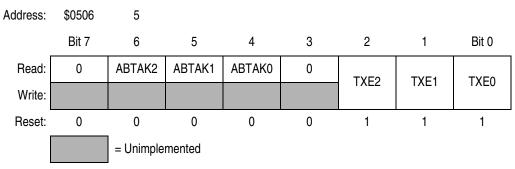
Figure 23-21. Transmitter Flag Register (CTFLG)
