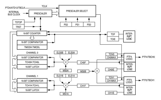
Figure 20-1. TIMB Block Diagram
