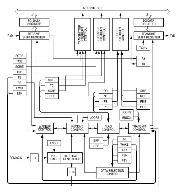
Figure 18-1. SCI Module Block Diagram
