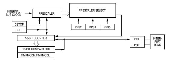
Figure 21-1. PIT Block Diagram
