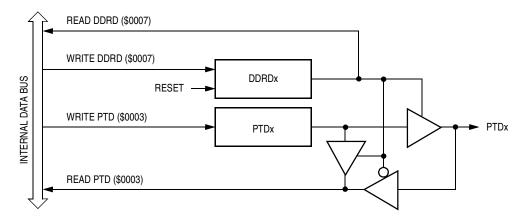
Figure 22-13. Port D I/O Circuit
