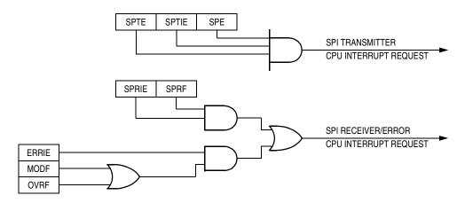
Figure 19-8. SPI Interrupt Request Generation
