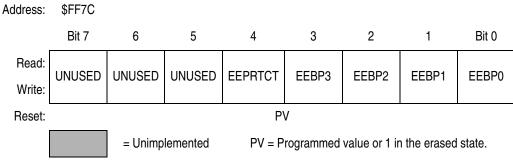
Figure 7-4. EEPROM-2 Nonvolatile Register (EE2NVR)
