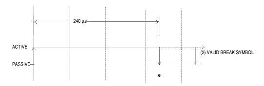
Figure 27-10. J1850 VPW Received BREAK Symbol Times
