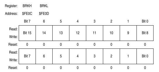
Figure 13-4. Break Address Registers (BRKH and BRKL)
