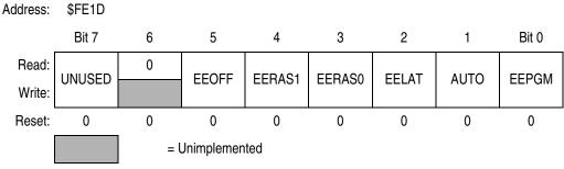
Figure 6-2. EEPROM-1 Control Register (EE1CR)
