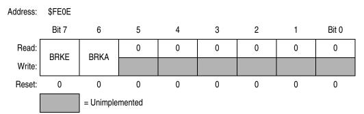
Figure 13-3. Break Status and Control Register (BSCR)
