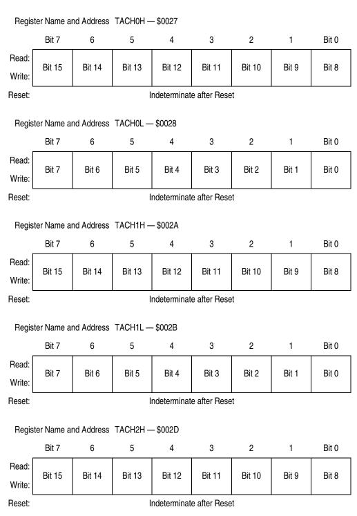
Figure 25-9. TIMA Channel Registers (TACH0H/L-TACH5H/L) (Sheet 1 of 3)
