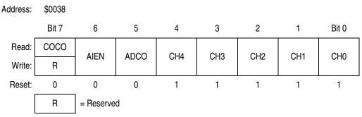
Figure 26-2. ADC Status and Control Register (ADSCR)
