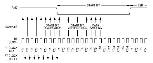
Figure 18-8. Receiver Data Sampling
