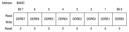
Figure 22-15. Data Direction Register E (DDRE)
