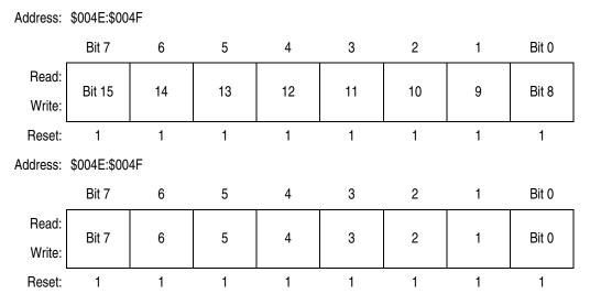
Figure 21-5. PIT Counter Modulo Registers (PMODH-PMODL)
