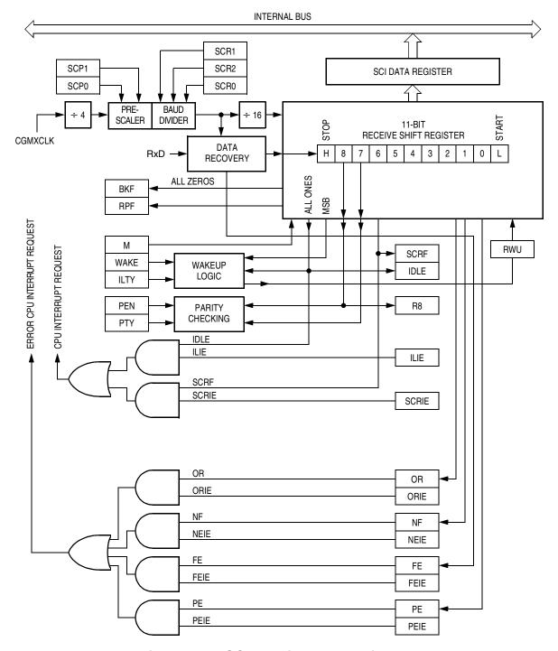
Figure 18-6. SCI Receiver Block Diagram
