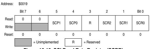
Figure 18-18. SCI Baud Rate Register (SCBR)
