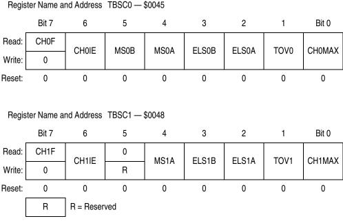
Figure 20-7. TIMB Channel Status and Control Registers (TBSC0–TBSC1)
