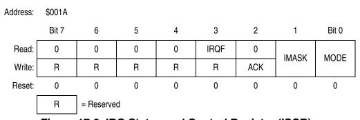
Figure 17-3. IRQ Status and Control Register (ISCR)
