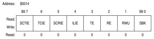
Figure 18-12. SCI Control Register 2 (SCC2)
