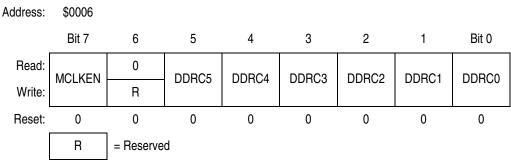
Figure 22-9. Data Direction Register C (DDRC)
