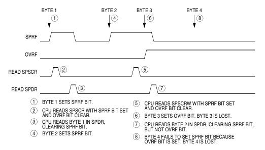
Figure 19-6. Missed Read of Overflow Condition
