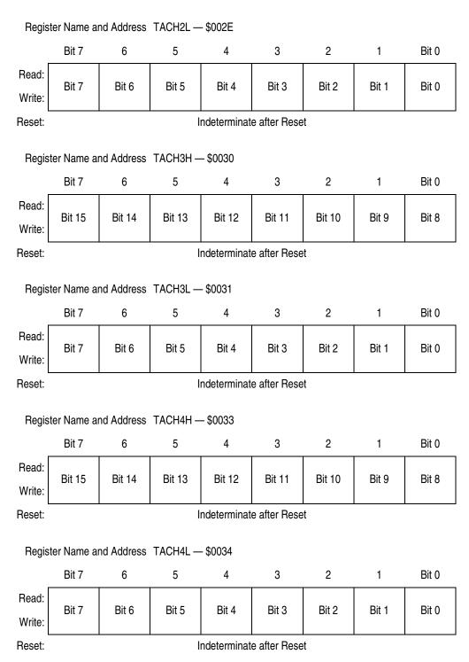
Figure 25-9. TIMA Channel Registers (TACH0H/L-TACH5H/L) (Sheet 2 of 3)
