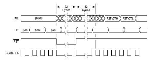
Figure 9-14. Wait Recovery from Internal Reset
