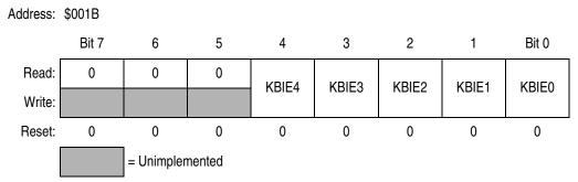
Figure 24-4. Keyboard Interrupt Enable Register (KBIER)
