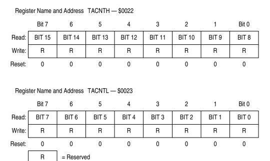
Figure 25-5. TIMA Counter Registers (TACNTH and TACNTL)
