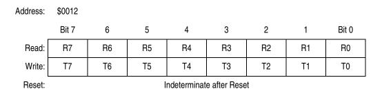
Figure 19-13. SPI Data Register (SPDR)
