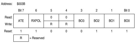
Figure 27-15. BDLC Analog and Roundtrip Delay Register (BARD)
