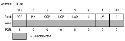
Figure 9-18. SIM Reset Status Register (SRSR)
