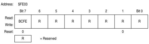
Figure 9-19. SIM Break Flag Control Register (SBFCR)
