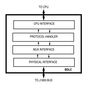
Figure 27-1. BDLC Block Diagram
