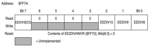
Figure 7-5. EE2DIV Divider High Register (EE2DIVH)
