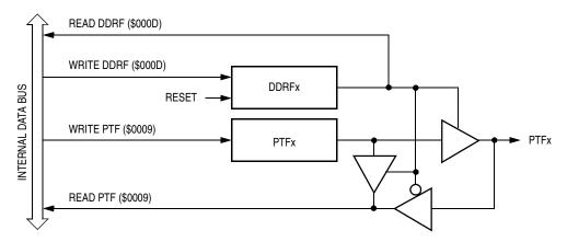
Figure 22-19. Port F I/O Circuit
