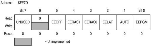
Figure 7-2. EEPROM-2 Control Register (EE2CR)
