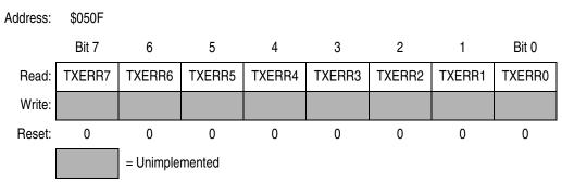
Figure 23-25. Transmit Error Counter (CTXERR)
