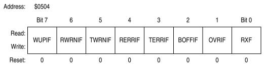
Figure 23-19. Receiver Flag Register (CRFLG)
