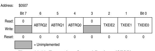
Figure 23-22. Transmitter Control Register (CTCR)
