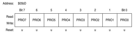
Figure 23-13. Transmit Buffer Priority Register (TBPR)
