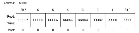
Figure 22-12. Data Direction Register D (DDRD)
