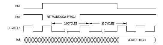
Figure 9-5. Internal Reset Timing
