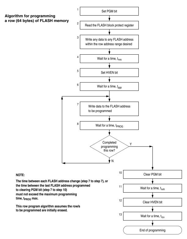
Figure 4-4. FLASH Programming Algorithm Flowchart
