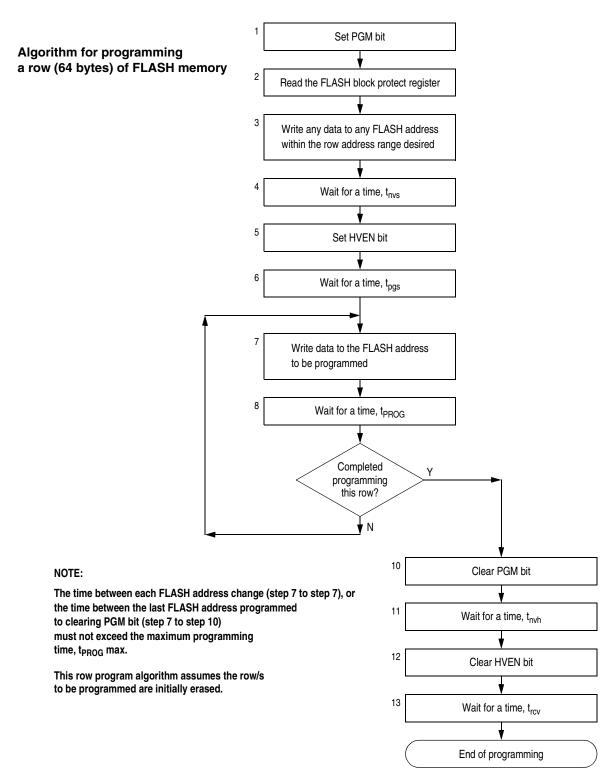
Figure 5-4. FLASH Programming Algorithm Flowchart
