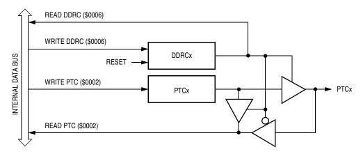
Figure 22-10. Port C I/O Circuit
