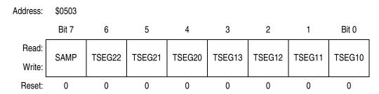
Figure 23-18. Bus Timing Register 1 (CBTR1)
