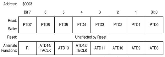
Figure 22-11. Port D Data Register (PTD)
