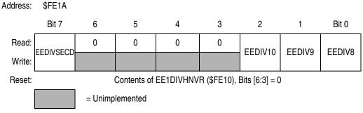
Figure 6-5. EE1DIV Divider High Register (EE1DIVH)
