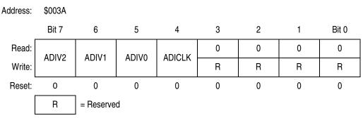
Figure 26-4. ADC Input Clock Register (ADICLK)
