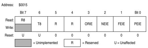
Figure 18-13. SCI Control Register 3 (SCC3)
