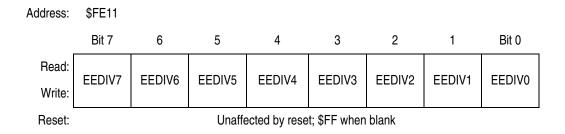
Figure 6-8. EEPROM-1 Divider Non-Volatile Register Low (EE1DIVLNVR)
