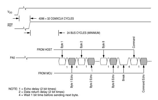
Figure 14-6. Monitor Mode Entry Timing
