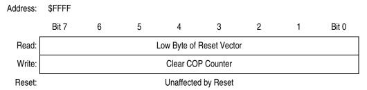
Figure 15-2. COP Control Register (COPCTL)
