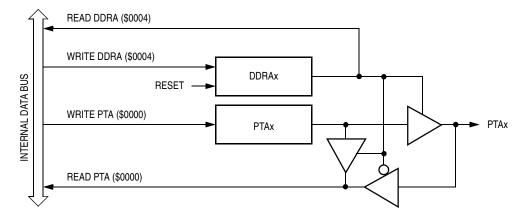
Figure 22-4. Port A I/O Circuit
