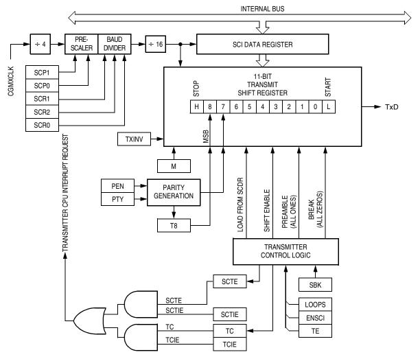
Figure 18-4. SCI Transmitter
