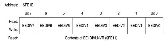
Figure 6-6. EE1DIV Divider Low Register (EE1DIVL)
