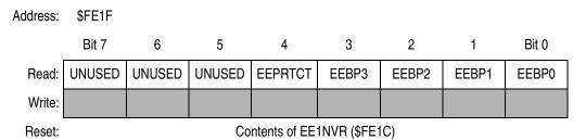
Figure 6-3. EEPROM-1 Array Configuration Register (EE1ACR)
