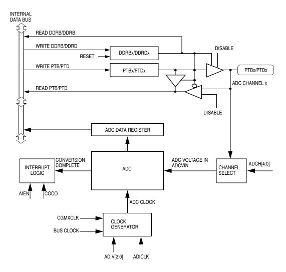
Figure 26-1. ADC Block Diagram
