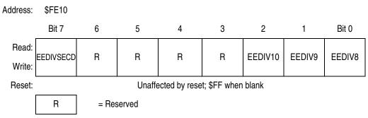
Figure 6-7. EEPROM-1 Divider Non-Volatile Register High (EE1DIVHNVR))
