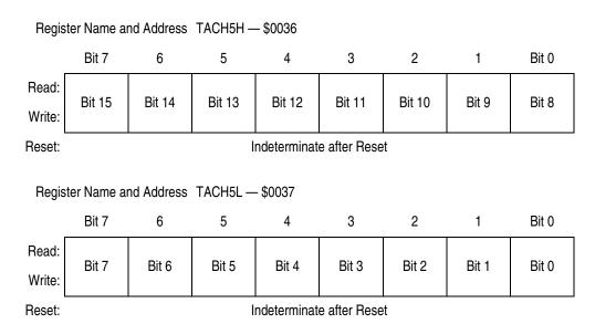
Figure 25-9. TIMA Channel Registers (TACH0H/L-TACH5H/L) (Sheet 3 of 3)
