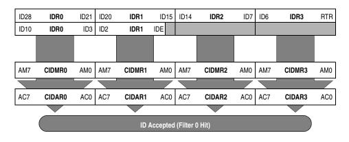
Figure 23-3. Single 32-Bit Maskable Identifier Acceptance Filter
