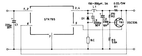
Unit (resistance:  $\Omega$ , capacitance: F)
