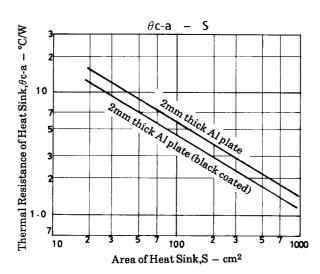
For 2mm thick Al plate (black coated), the area is  $30\text{cm}^2$ .  $(55\times55\times2t)$
