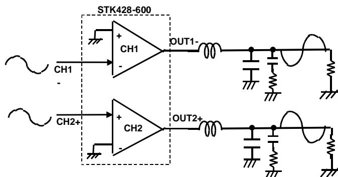
Synchronous signal 400 ~ 500kHz
