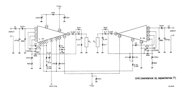
Equivalent Circuit Sample Application Circuit: 2-Channel 80 W min AF Power Amplifier
