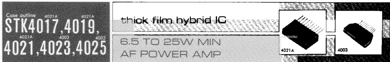
Fabricated on the IMST substrate of our own originality and designed for use in intermediate-power, single-channel, single-supply voltage amplifiers. Their packages are made much more compact than those of the Type Nos. heretofore in use, thereby meeting the requirements for making the set smaller and slimmer. They are especially suited for use in electronic organs or electric pianos.
