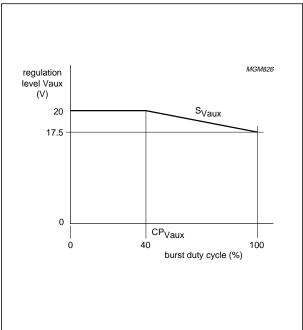
Fig.6 Regulation level V<sub>Vaux</sub> versus burst duty cycle.
