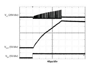
Typical Waveforms at  $V_{IN} = 5.5V$
