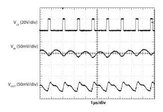
**Waveforms During Over-Voltage Protection**
