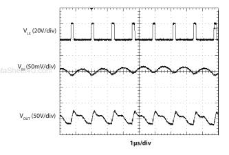
Typical Waveforms at  $V_{IN} = 3.6V$
